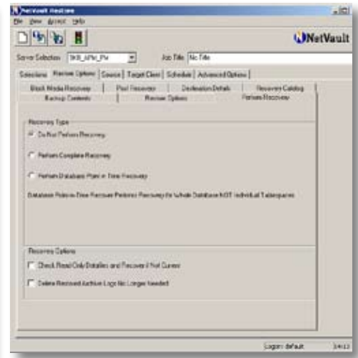
Figure 2. The NetVault: Backup APM for Oracle point-and-click interface speeds restores by eliminating the chance of syntax errors that would require a restart.
